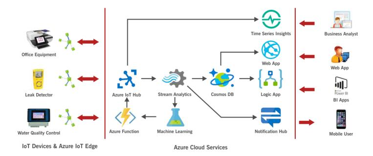
Figure 3. Typical Azure IoT Hub Solution
