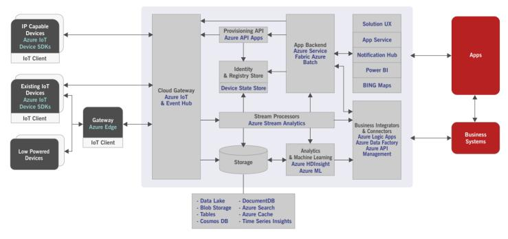
Figure 2. Azure IoT Hub Architecture
