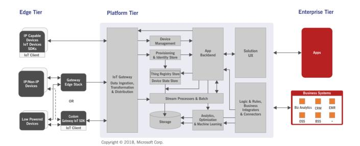
Figure 1. Typical 3-tier IoT Reference Architecture
